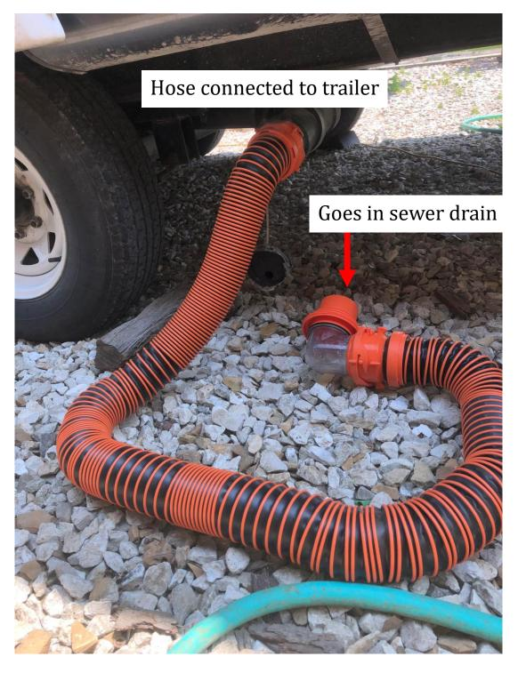
· If at a full-service camp site, connect the sewage discharge hose (stored in the black tube on lower front of trailer) to the trailer and the site sewer
