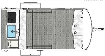
Dry Weight 1,775 - 1,850 lbs GVWR 2,200 lbs Net Carrying Capacity 400 - 550 lbs Ball Height 19" Fresh Water Tank 8.5 Gal" Exterior Frame All-Aluminum / All-Tube / Cage Frame
