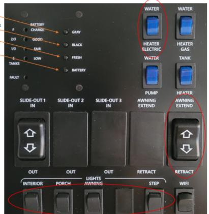
The electric water heater may remain on IF connected to city water and you are within the campground. When leaving the campground for extended periods of time please turn switch off (indicated by light being off as shown in this photo) and turn water supply off as well
