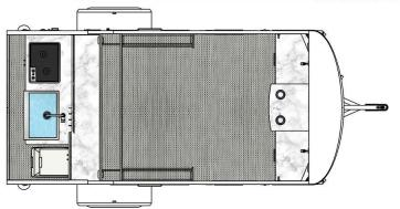
Dry Weight 1,775 - 1,850 lbs GVWR 2,200 lbs Net Carrying Capacity 400 - 550 lbs Ball Height 19" Fresh Water Tank 8.5 Gal" Exterior
